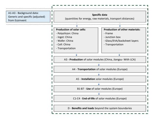
The PolySi, ingots, wafers, cells and modules are manufactured in China. The supply chain is shown below:
