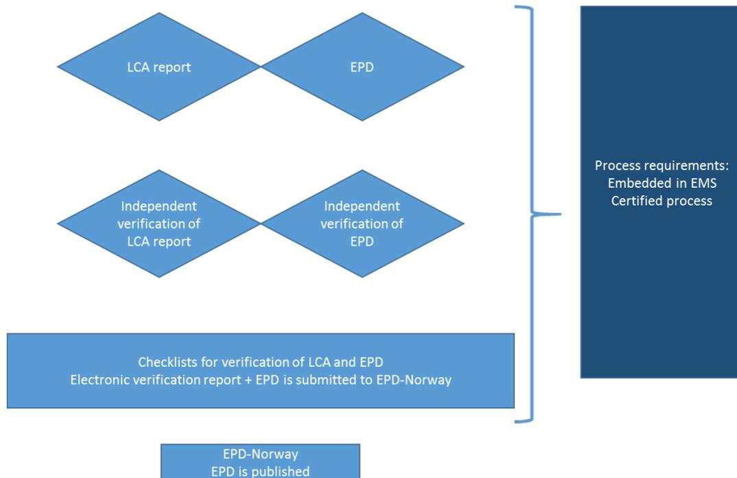
**Figure 4: Process certification tool**
