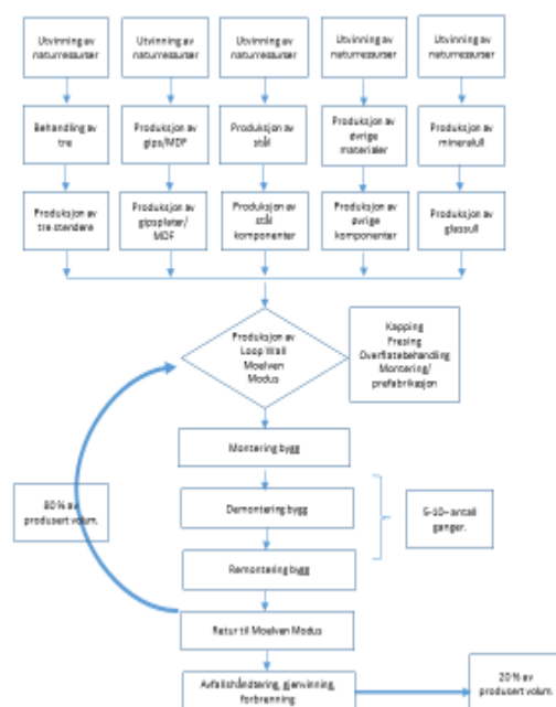
Figure 1. Flow diagram for the production of Loop Wall 300 - MDF system
