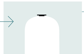
Welding of boss to liner
